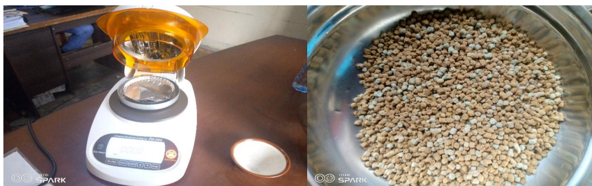
Figure 3: Infrared Moisture Analyzer FD-660(left) and a poorly dried fish feed (right)
