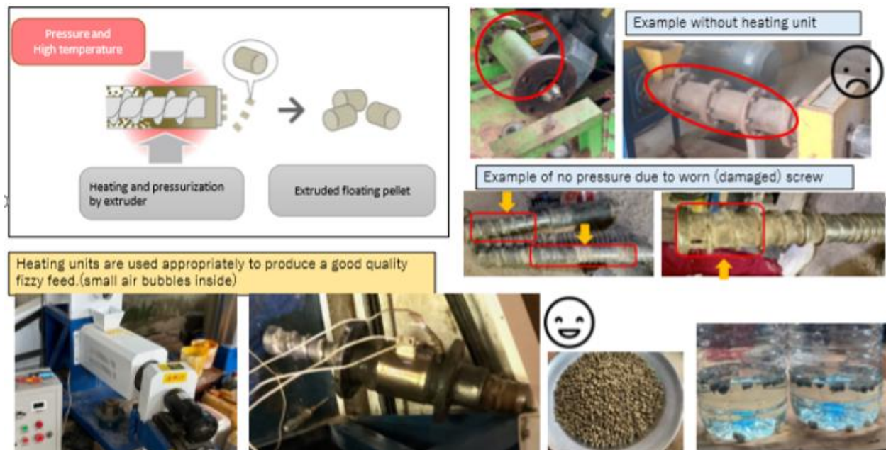
Figure 8: Appropriate and inappropriate temperature and pressure treatment during extrusion molding in floating fish feed formulation.
